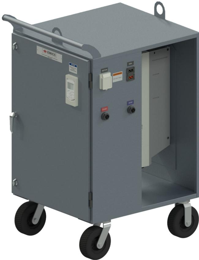
**The ALT-P series power carts are built to take a standard single phase 240 Volt generator and allow you to run a three phase pump motor up to 20 hp or rating of the generator and cart. This cart is built to run one pump, bypassing the pump control station all together. Providing extended running capability after severe storms and power failures.**
